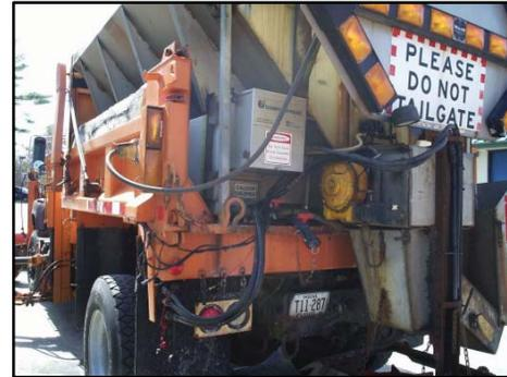
**What are the planning or technical considerations?** Overall costs will depend on the type of spreader controls selected. Although initially more expensive, serious consideration should be given to automated spreader controls due to their ability to save money on materials because material is being supplied appropriately.
