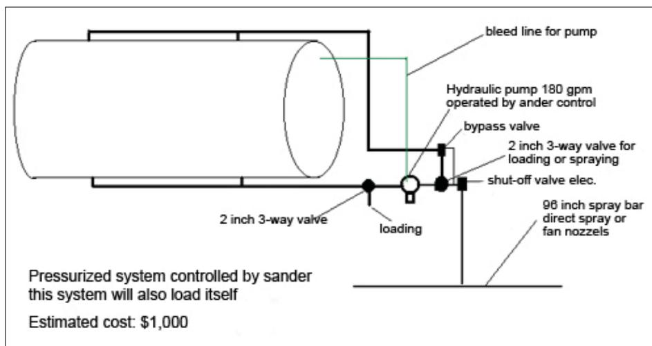
*Schematic of a Typical Pressurized System*
