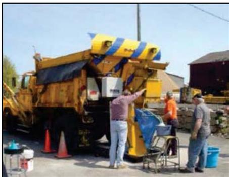
**What is it?** Calibration is an important procedure and involves adjusting the spreader to apply known amounts of material at specific settings. A snow fighter needs to be confident that a spreader is delivering the specific amount of material requested. Regular calibration ensures that this will happen.
